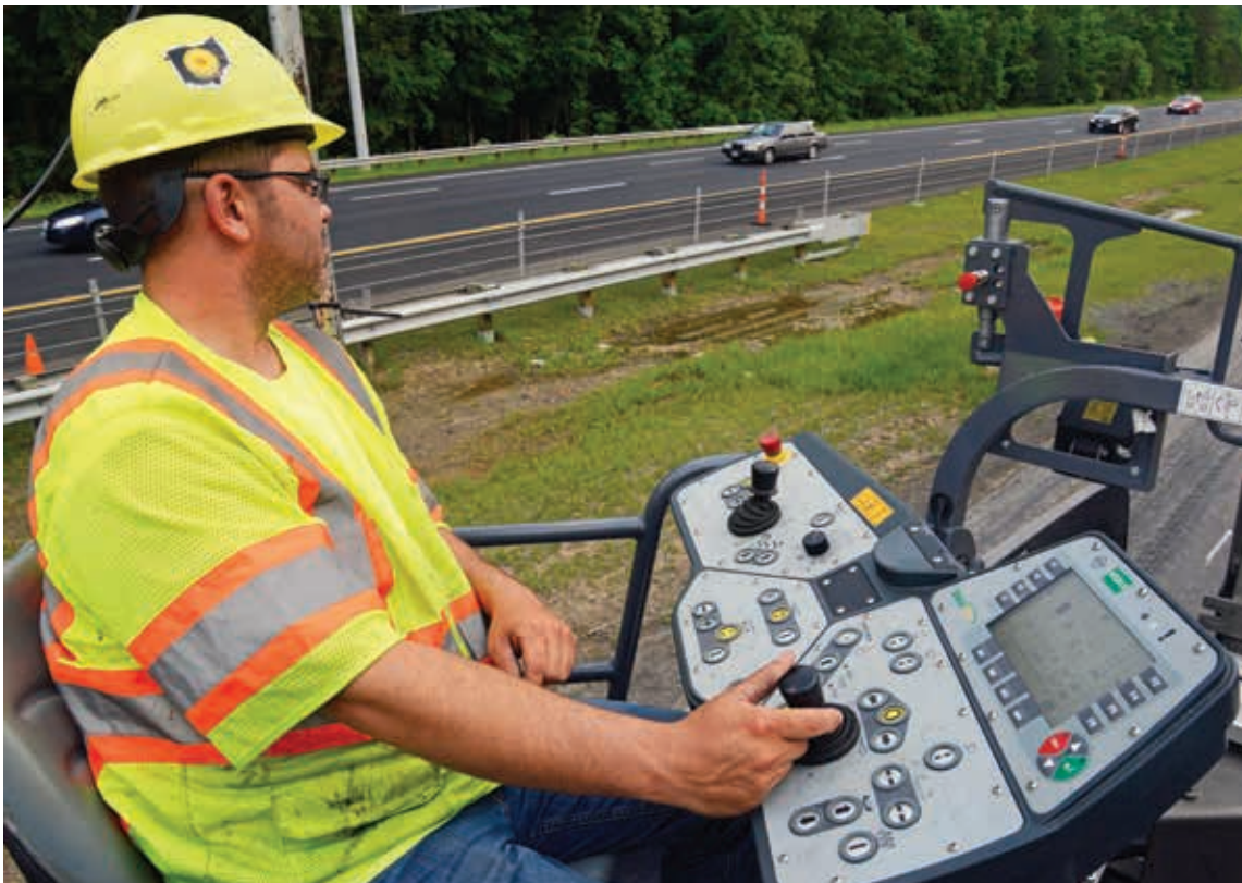
MT 3000-3i operator platform provides superb visibility into receiving hopper and pavement below
